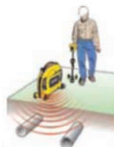
Induce a signal to locate utilities.
