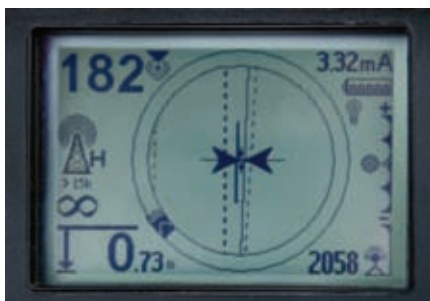
Screen in Omniseek mode: See multiple lines (Screenshot shows three different lines) ①, ②, ③.
