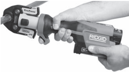
Figure 9 – Sertissage du raccord
