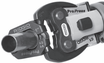
Figure 10 – Attaching Actuator to Press Ring
