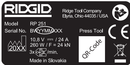
Figure 2 – Machine Serial Number - Circled digits indicate the year and month of the manufacture. (YY = year, MM = month,)
