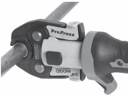
Figure 7 – Placing Scissor-Style Jaws Around Fitting
