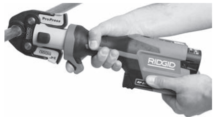
Figure 9 – Pressing the Fitting
