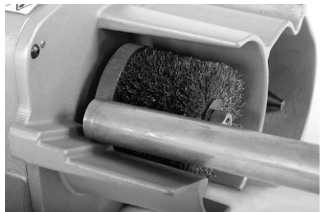
Figure 12 – Deburring O.D. Of Tube
