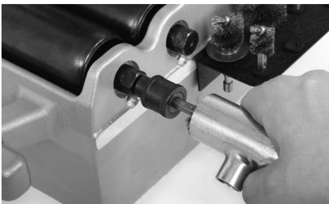
Figure 14 – Nettoyage interne des raccords
