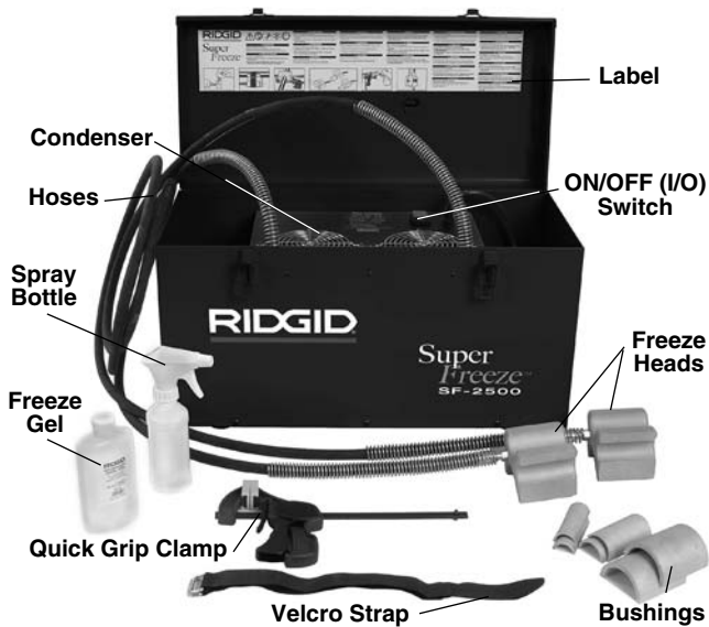
Figure 1 – SF-2500 SuperFreeze Unit
